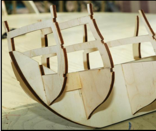
Figure 10: Bow Frames in Position
