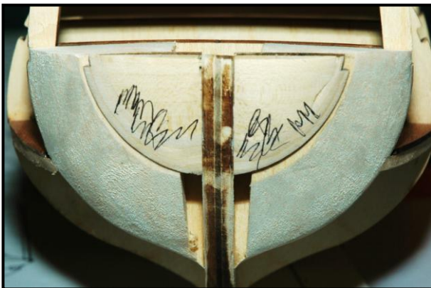
Figure 31: Partially Shaped Bow Filler Blocks
