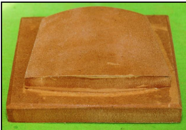
Figure 71: Base Board Used to Create Curved Transom
