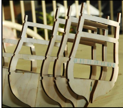
Figure 10: Stern Frames in Position
