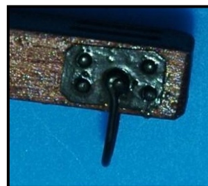
Figure 89: Curved Cathead Showing Bracket for Anchor Stowage
