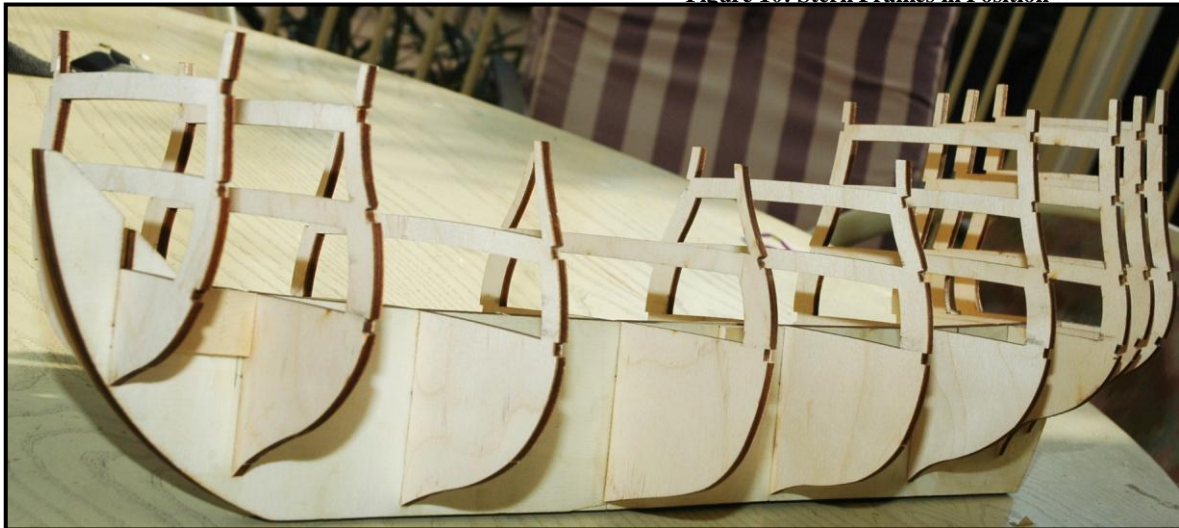
Figure 11: Overall View of Frames in Position
