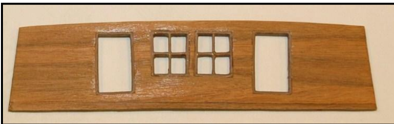
Figure 41: First Stage of Building Bulkhead B
