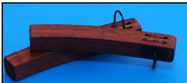
Figure 89: Curved Cathead Showing Bracket for Anchor Stowage
