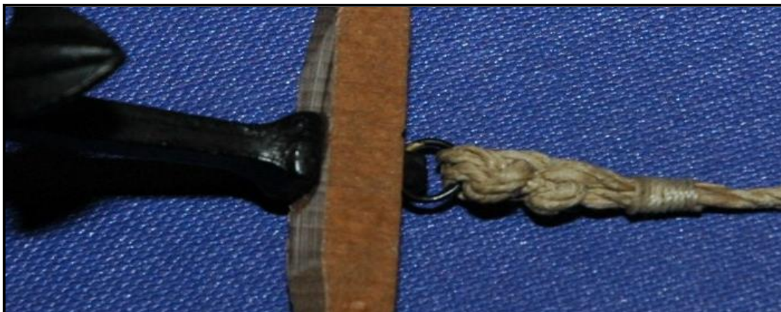
Figure 62: Anchor Rigging Showing Fisherman's Knot
