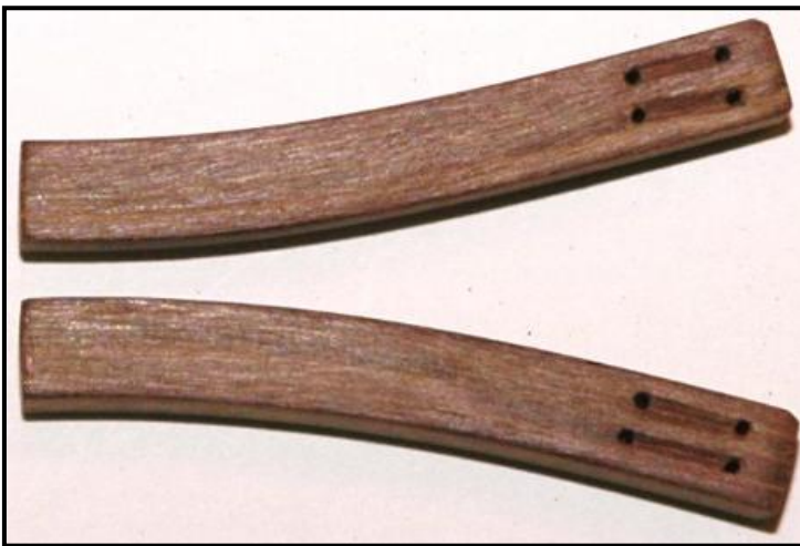
Figure 66: Sheaves in the Curved Catheads
