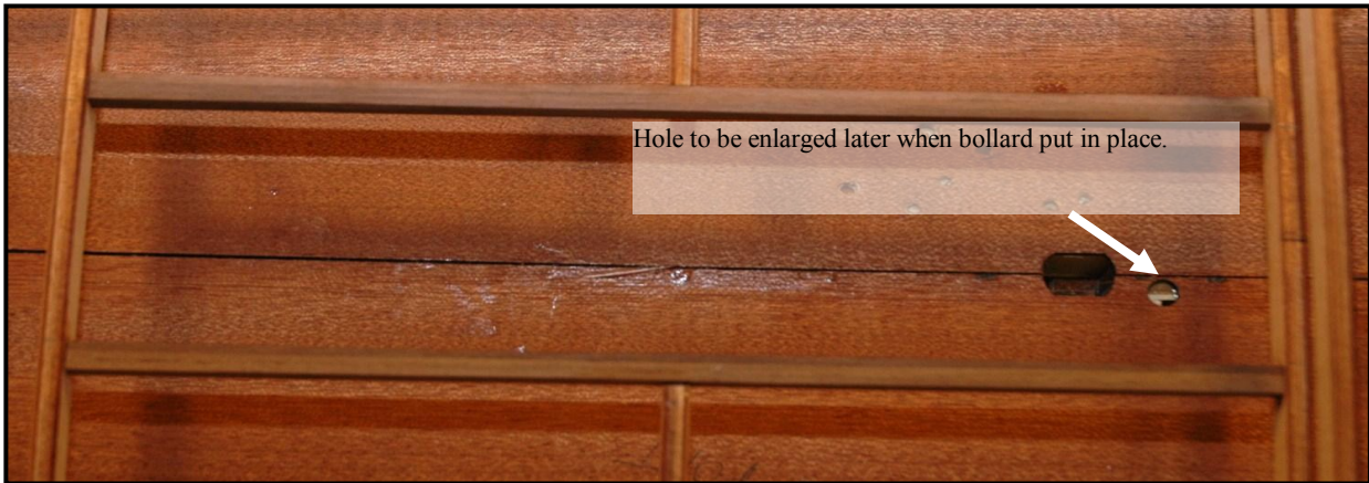
Figure 22: Enlargement of Deck Opening for Bollard
