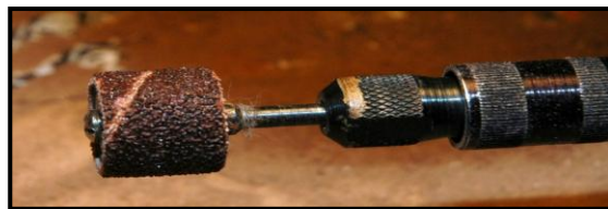
Dremel tools (high speed cutter tool, sanding drum & other bits; flexible drive attachment; along with a mini drill press )
