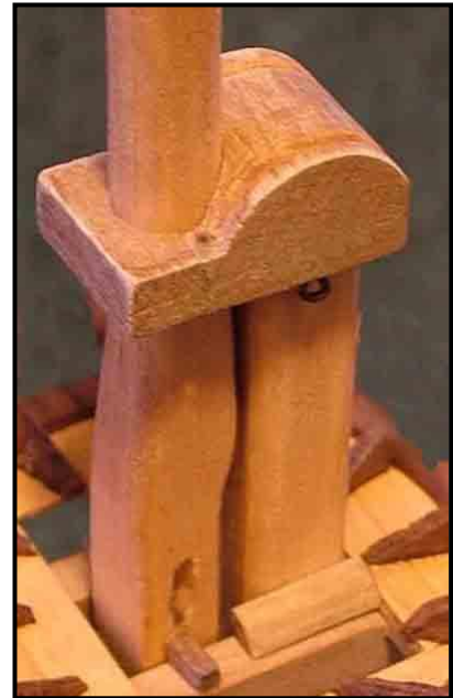
Figure 42: Advanced Topmast Heel A quandary occurs at this point – as it does with other similar mast sections. The rounded mast below the head is finished at 6.0 mm. diameter and so the minimum finished width of the head above it must be 6.0 mm. to fit. Mathematically, it follows that this would be formed from a rod with a minimum diameter of 8.48 mm. The original rod diameter in the kit varied considerably from 7.90 – 8.17 mm. in diameter.
