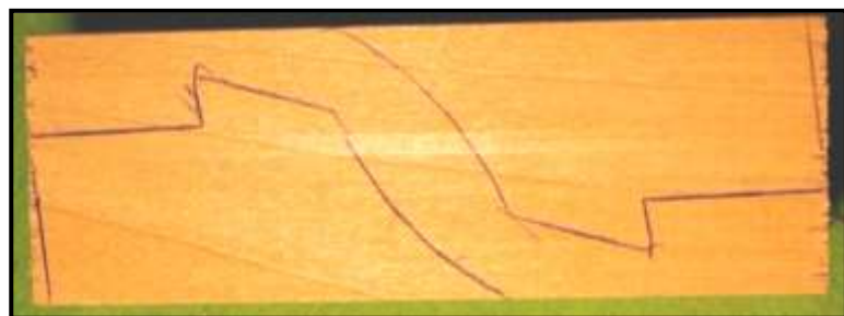
Figure 9: Marking Out Two Filler Blocks
