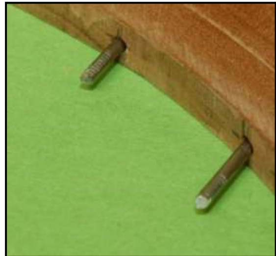
Figure 83: Supporting Nails for Stem Post
