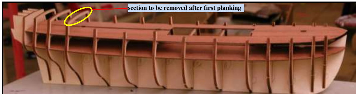
Figure 7: All Transverse Frames in Position
