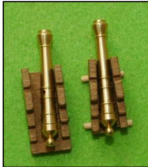
Figure 53: Difference Between 'Square' and a 'Tapered' Gun Carriage
