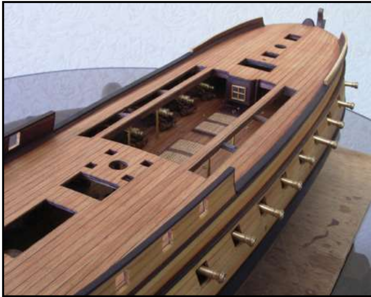
Figure 25: Full-length Timbers Used for Planking
