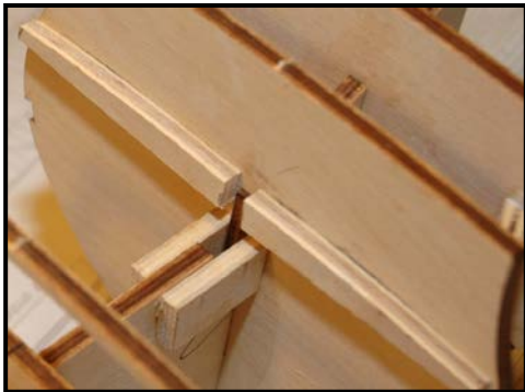
Figure 14: Deck Support Glued onto Frame C
