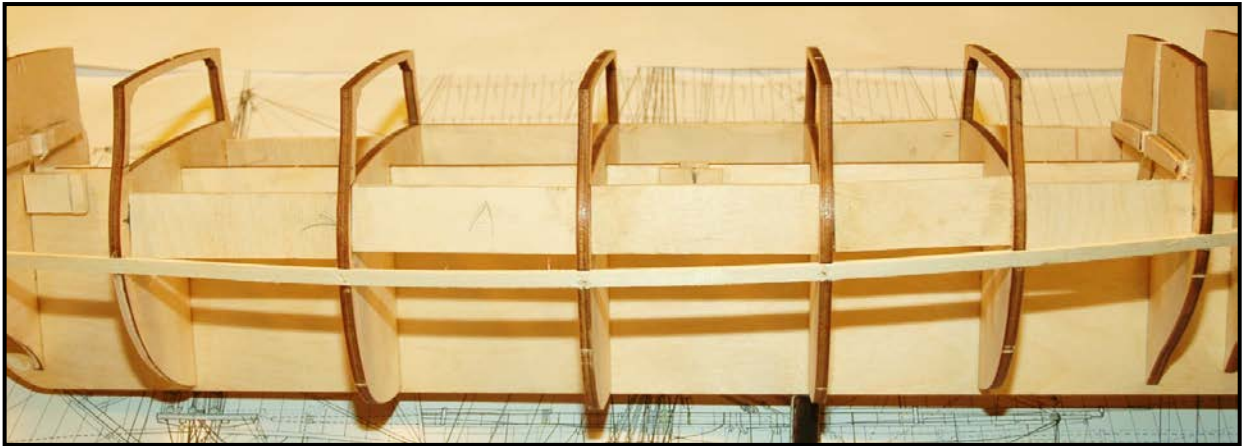
Figure 19: Longitudinal Stringers in Position
