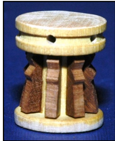
Figure 49: Typical Form for Both Capstans
