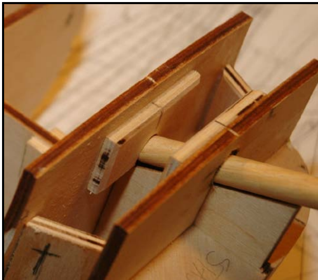
Figure 20: Creating Support for Bowsprit
