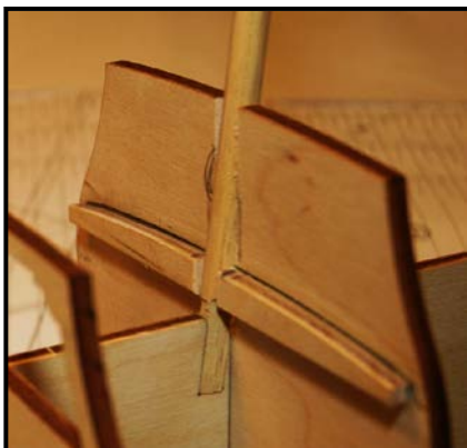
Figure 16: Slot Cut into Frame 3
