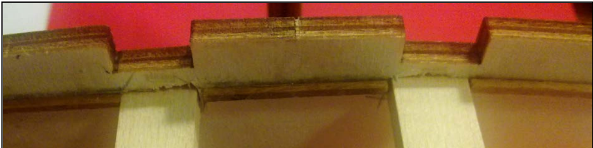
Figure 13: Main Deck End Supports
