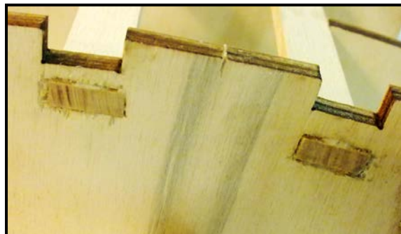
Figure 11: Holes Cut Into Frame 6 For Longitudinal
