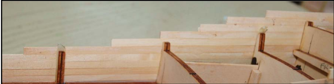
Figure 47: First Planking at Various Stages (cont.)
