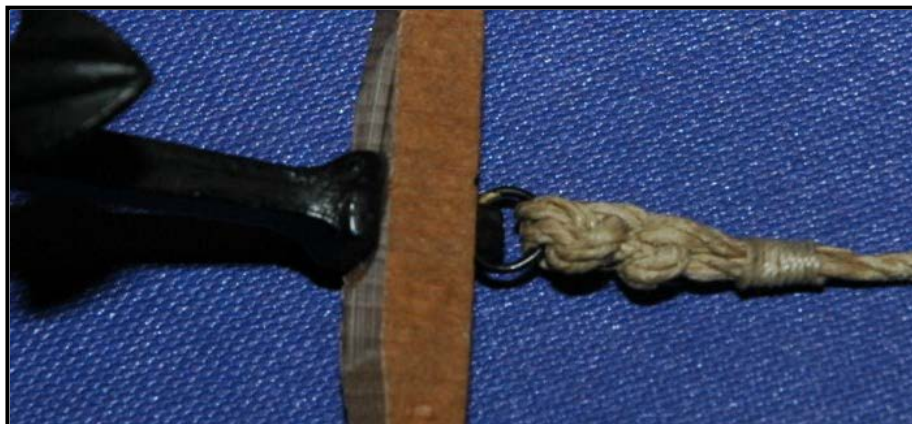
Figure 34: Anchor Rigging Showing Fisherman's Knot
