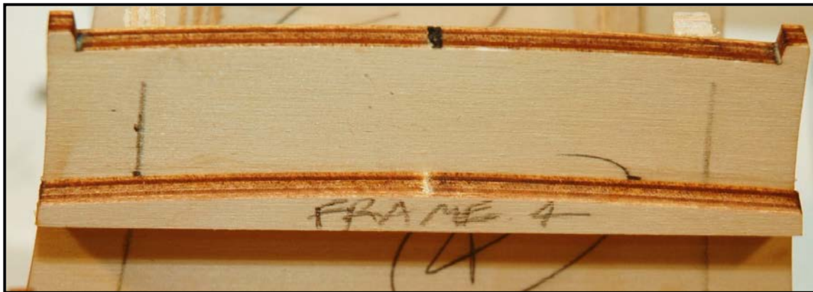
Figure 9: Adding Deck Formers to Support Decking
