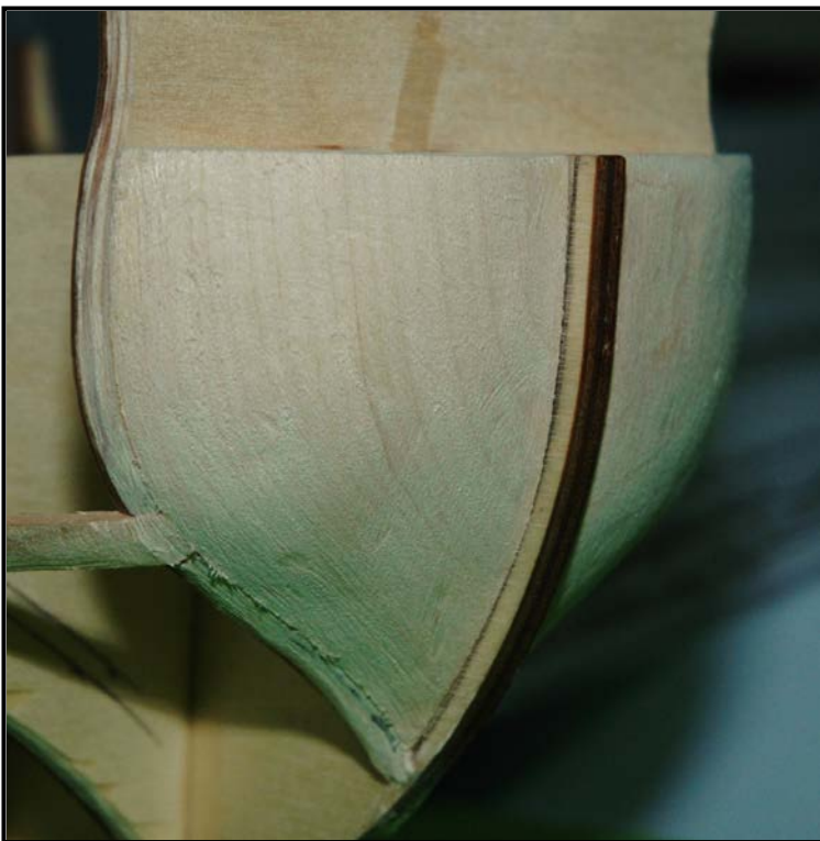
Figure 15: Bow Filler Blocks in Position
