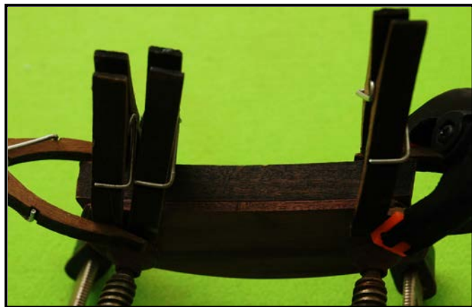
Figure 21: Forcing Shape of Transom Support Piece 'B' one side until the first planking was complete. Be warned – some modification is required on this transom support...' Control+ Click' on Side Gallery Positioning
