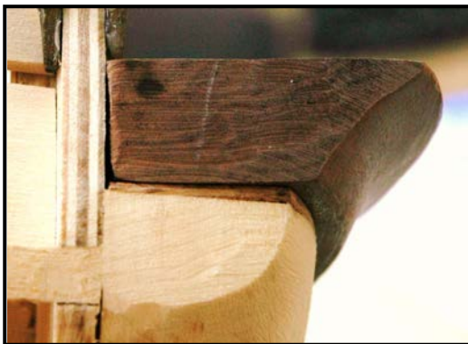
Figure 22: Checking Fit of Transom Support Piece 'C'
