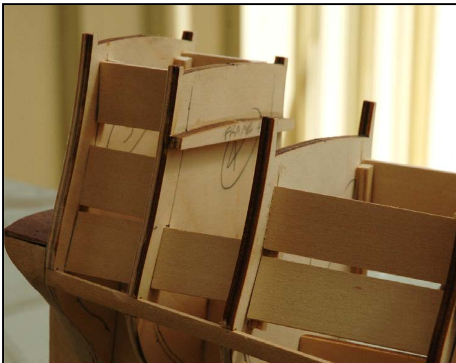
Figure 11: Adding Gun Support Timbers
