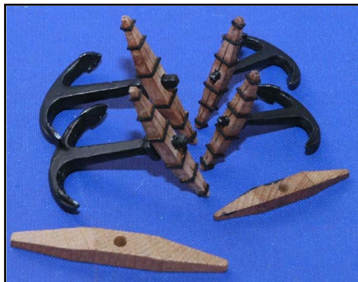
Figure 75: Anchors Complete With Metal Hoops; Stocks Supplied But Not Utilised
