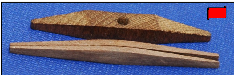
Figure 74: Underside View of Partially Completed Stock of Bow Anchor; Advanced
