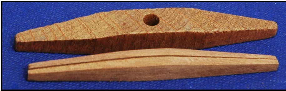
Figure 70: Underside View of Partially Completed Stock of Sheet Anchor; Advanced
