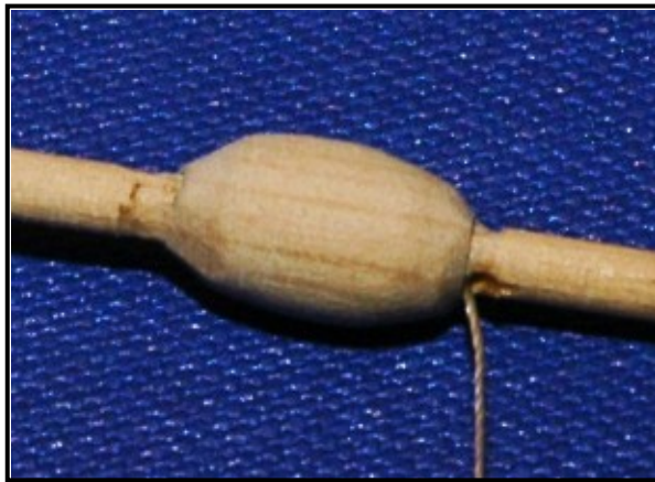
Figure 55: Fixing the Rope into the Buoy
