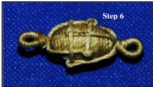
Figure 57: Steps in Rigging a Buoy
