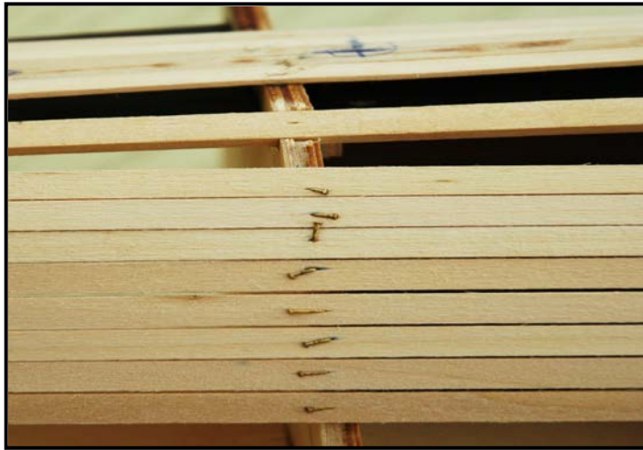
Figure 43: First Planking Shrinkage
