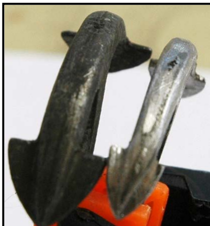
Figure 52: Reducing Fluke Size & Overall Width of Anchor
