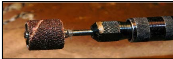
Dremel tools (high speed cutter tool, sanding drum & other bits; flexible drive attachment; along with a mini drill )
