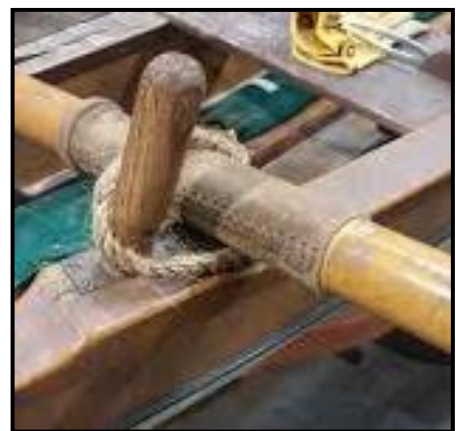
Figure 26: Oar Lashed to a Tholepin
