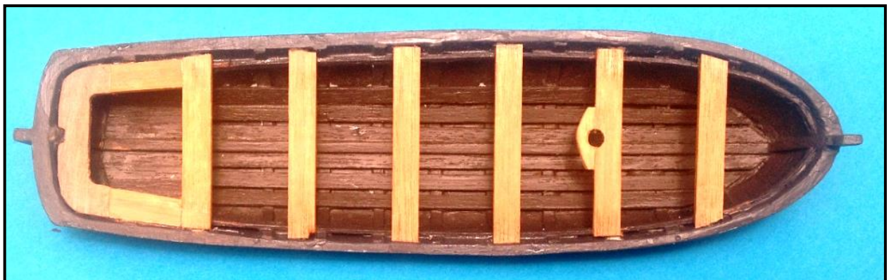
Figure 20: Thwarts & Sheets Installed in Barge
