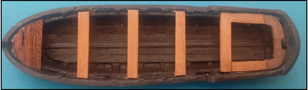
Figure 21: Thwarts & Sheets Installed in Cutter
