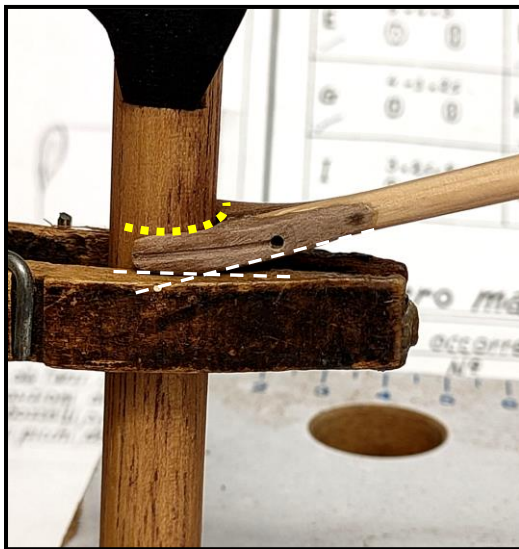
Figure 12: Checking Alignment & Mast Fit
