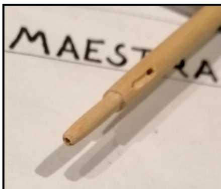
Figure 14: Iron Hole, Aft End of Spanker Gaff
