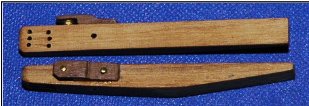
Figure 31: Cathead with Fourth Sheave
