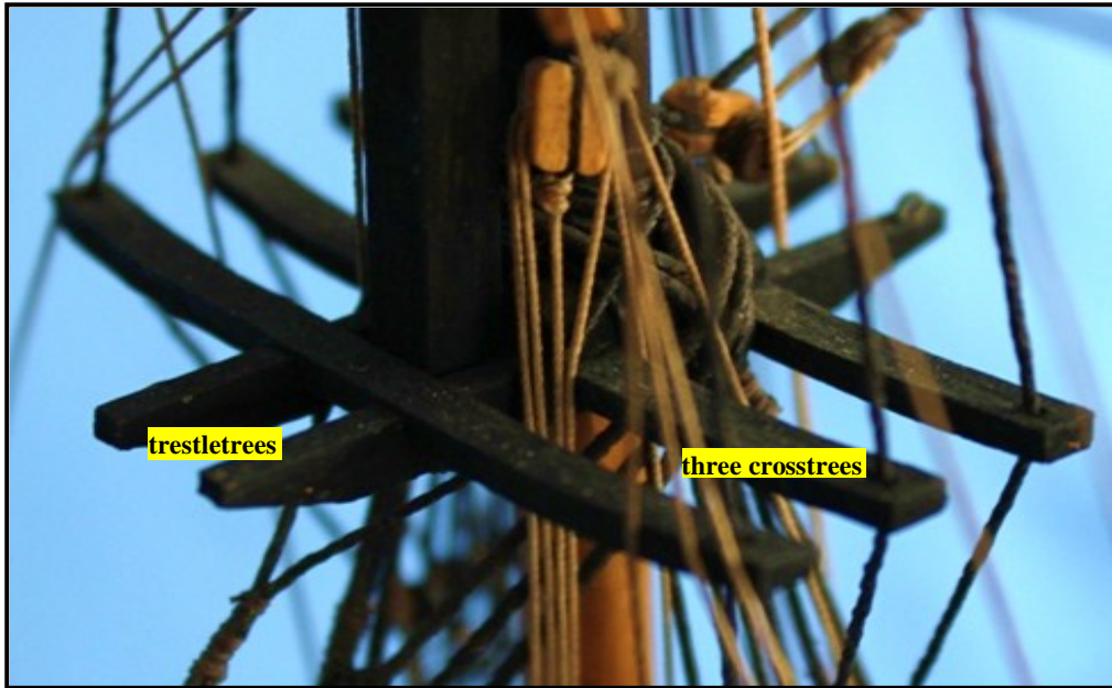
Figure 10: Typical Crosstree/ Trestletree Frame
