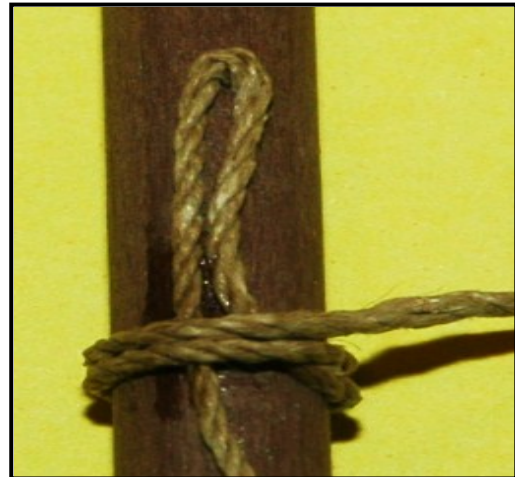
Figure 15: Beginning Woolding Serving
