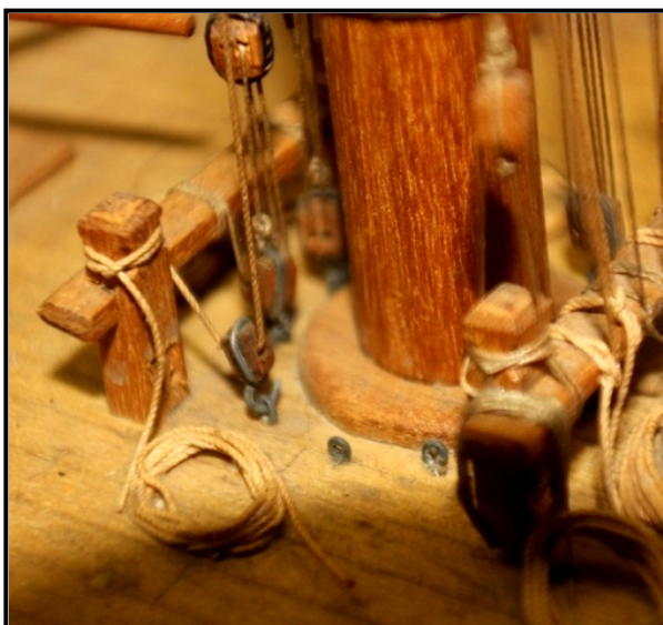
Figure 19: Main Mast Collar
