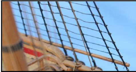
Figure 17: Photographic View of Ratlines
