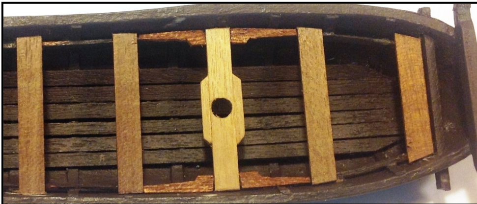
Figure 30: Reinforcement of Mast-Supporting Thwart
