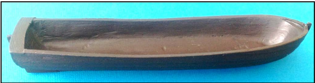
Figure 11: Wet Brush Layer
