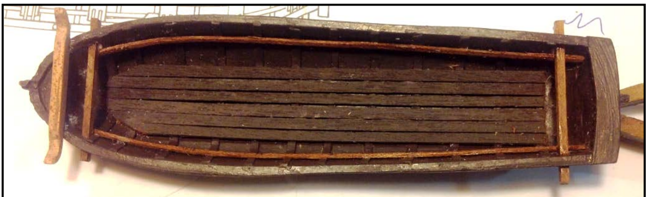
Figure 18: Kedging Bars (fore and aft)
