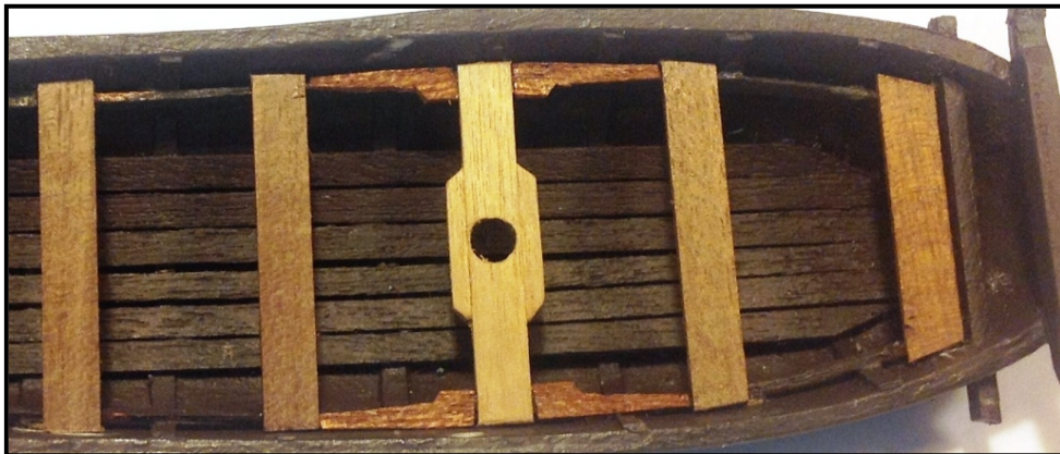
Figure 20: Reinforcement of Mast-Supporting Thwart
