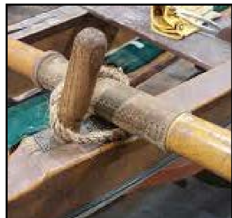
Figure 21: Oar Lashed to a Tholepin
