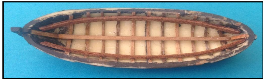
Figure 21: Ribs, Keel & Risers in the Service Boat
