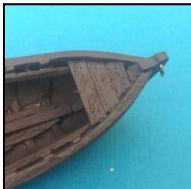
Figure 24: Construction of Boat Head Sheets
