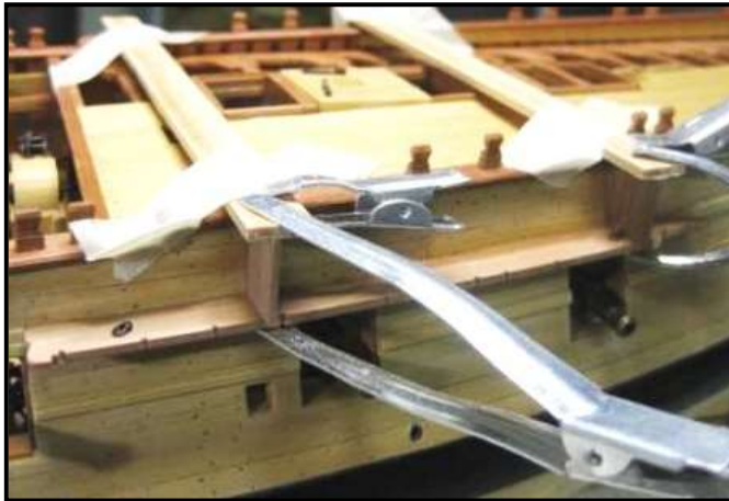
Figure 32: Holding Channels in Correct Alignment
