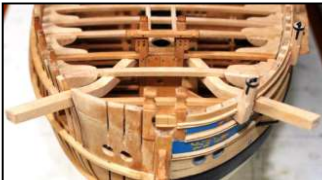
Figure 26: Underlaid Diagonal Fastening
