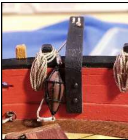
Figure 22: Vertical Fastening (on smaller ships)
