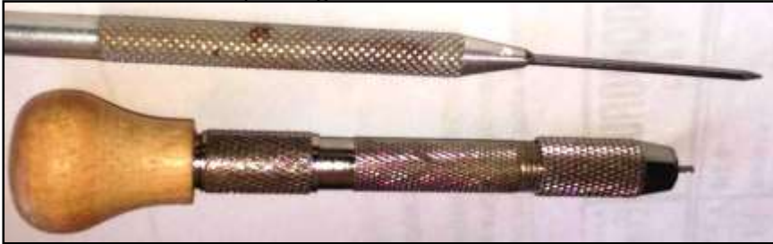
Figure 18: Pointed Punch (above) & Pin Vice (below)
