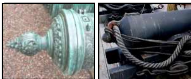
Figure 22: Breeching Spliced to Cascabel ... or Passed Through a Ring
