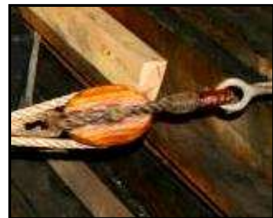
Figure 27: Block Splicing to Ringbolt
